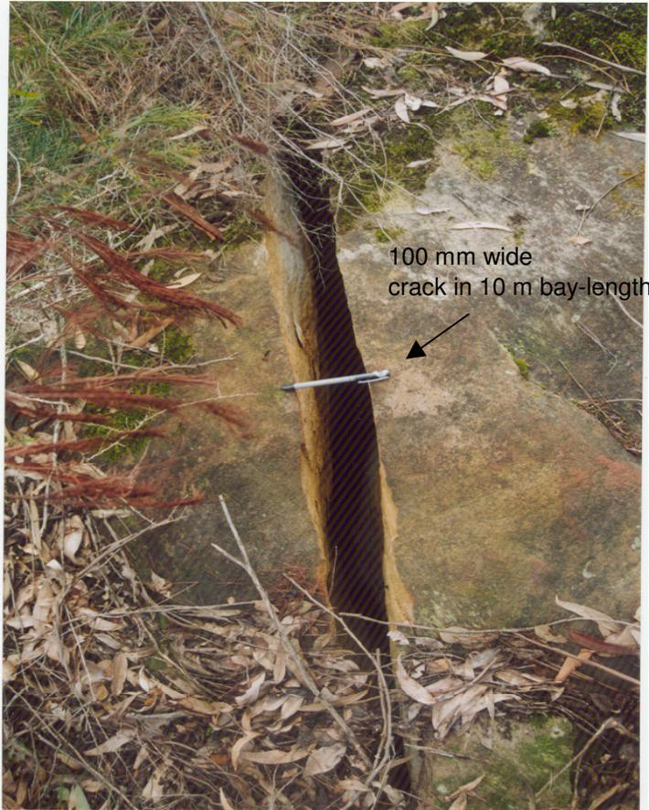
Strain Concentration Factor Calculation for 10 m Baylength<sup>^</sup>
